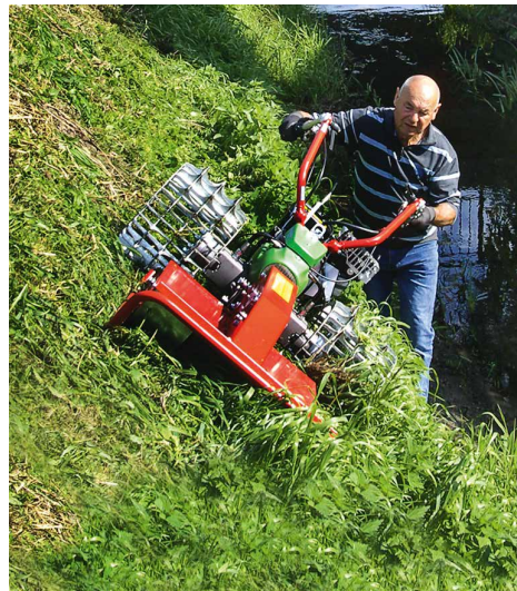
Robust, 8 mm thick steel blades
