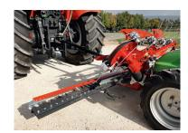
Transport to the place of operation The entire combination can also be moved over long distances to the place of operation with a tractor using the drawbar. The freewheeling setting of the single-axle walkbehind tractor is used in this case.
