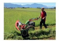
The Rapid Compact zero grazers are mounted on the walk-behind tractor and are designed for picking up green forage.
