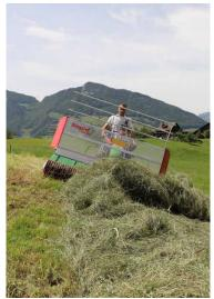
The Rapid Multi-Twister has a conveyor belt with which the crop is actively transported to the side after being collected by the well-tried pick-up. Deployment on slopes and on level surfaces is therefore possible. Furthermore, the active discharge increases the range of uses with regard to green forage and silage. The conveyor belt also makes the «swathe» work operation possible from a procedural point of view.
