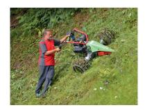
With the Rapid REX you can now carry out work that was once the preserve of scythes. Weighing just 85 kg and featuring a low centre of gravity, it can be used to tackle slopes with a gradient of up to 120% safely. The active handlebar steering means that it can be manoeuvred safely, precisely and with ease even on challenging terrain.
