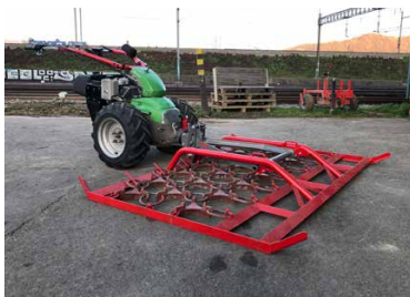
Towed attachment Due to the conceptual structure of the pasture harrow, it is possible to work comfortably trailing/pulling in the forward direction.
