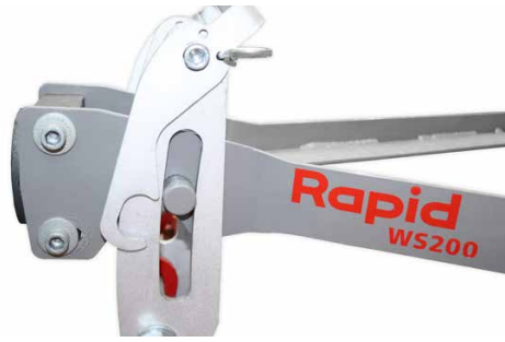
In working position, pasture harrow floating
