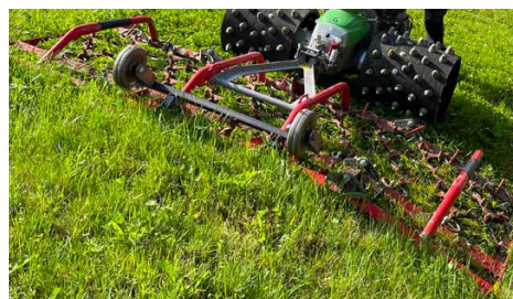
The multi-piece frame version offers additional properties. During application, the individual frame sections adapt well to the terrain, even on hilly surfaces.
