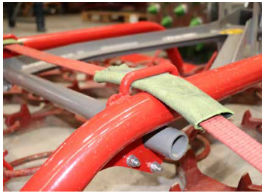
Lifting, loading, securing Crane eyelets and tabs for threading tension belts enable easy hanging and reliable load securing.
