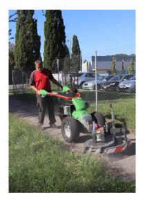
Edges, sides and paved areas are freed from weeds with the weed brush. The cleanliness, safety and protection of structures is thereby maintained. At pavement edges and gutters, drainage functions are retained and the accumulation of sediment is avoided. The procedure uses a mechanical method to pull up the weeds in different directions and deposit them on the surface.
