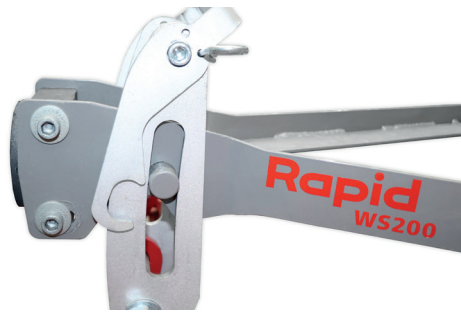
In working position, pasture harrow floating
