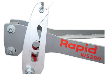
In transport or loading position, pasture harrow fixed
