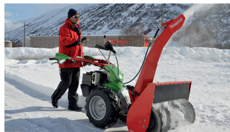
Target location for snow throwing can be conveniently adjusted via the handlebar during travel
